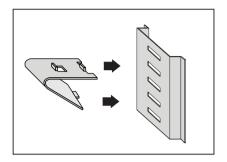
1. Some models come standard with shelves, shelf clips and notched pilasters. Each shelf requires four clips. Attach the shelf clips onto the pilasters by inserting its top hook into a pilaster notch followed by the bottom hook. Do not use pliers or other crimping tools to modify the shape of the shelf clips. This will result in shelf mounting instability.
