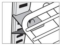
2. Place shelves on the shelf clips making sure all corners are mounted securely and evenly with identical distance from the unit's floor and up. Always lay the back of each shelf down on the rear clips before the front.
