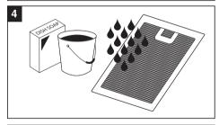
**4.** Wash the condenser coil air filter with luke warm water and dish soap. Rinse thoroughly and allow to dry.
