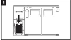
**5.** Re-insert the condenser coil air filter in the holding brackets.
