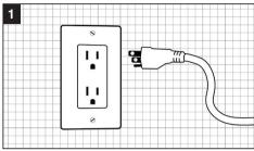
**1.** Disconnect the unit from the outlet before performing maintenance.
