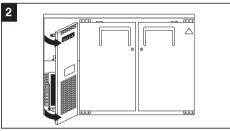
2. Locate the condenser coil panel door at the front, left side of the unit. Swing open the panel door to access the condenser coil air filter. The condenser coil air filter is a black rectangular, leather-framed mesh fabric mounted at either of the following locations: inserted behind the vents of the panel door or attached directly in front of the condenser coil.
